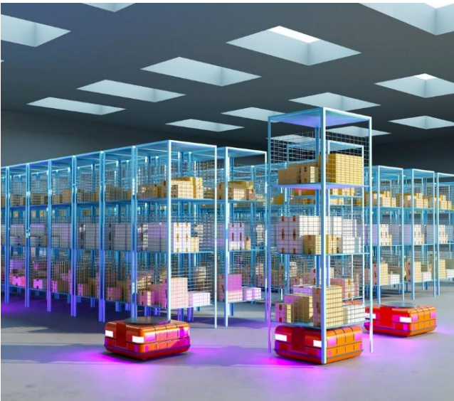
Figure 2. Automated guided vehicles (AGCs) being used to move materials in a warehouse
